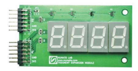
Seven segment LED display expansion module feature four 7-segment LED displays. This expansion module is designed to be directly compatible with FPGA/Micro-controller development boards featuring a 2×6 pin Expansion connectors. This module can still be used with other boards by using manual wiring. The heart of the board is four Common Anode high brightness LED display blocks. Segment multiplexing allows this module to operate with as small as 12 GPIOs.
