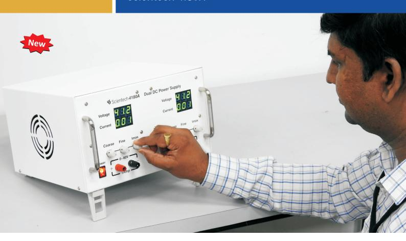
Scientech 4180A Dual DC Power Supply is designed as a Constant Current (CC) and Constant Voltage (CV) source for use in laboratories, industries and field testing. With compact size, light weight and low Power loss, it provides DC output voltages for Analog and Digital testing.
