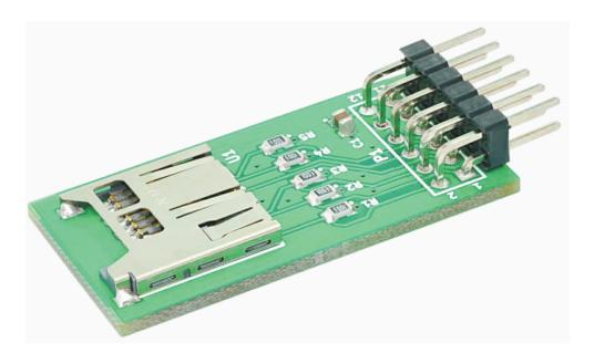
Micro SD Expansion Module provides an easy and convenient way to interface the Micro SD card to Numato Lab's FPGA/Microcontroller boards. It can be connected to any FPGA/Microcontroller board featuring a 2×6 pin Expansion connector. This module can be manually wired to FPGA/Microcontroller boards that do not have a 2×6 expansion header. This product is compatible with most of the Numato Lab's FPGA boards.
