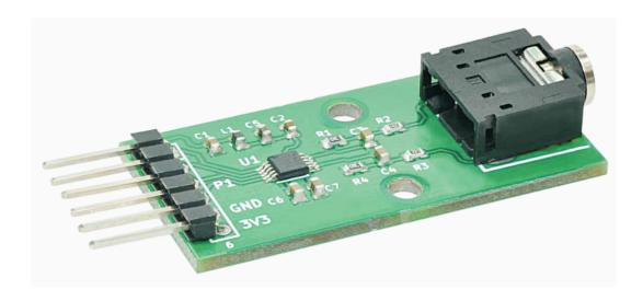
This module features 24-Bit, 192 kHz Stereo D/A Converter that enables producing high-quality stereo audio from a digital source. It supports all major audio data interface formats. This module is designed to be used with FPGA/Microcontroller boards featuring a 2×6 pin Expansion connector. It can also be used with other boards and connector types by using manual wiring. This product is compatible with most of the Numato Lab's FPGA boards.
