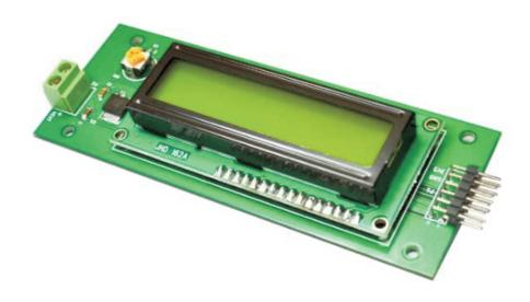
This expansion module features a 16×2 Alphanumeric LCD Module which can be added to your custom project using a 2×6 pin connector. It is designed to be used with Numato Lab's FPGA/Microcontroller boards featuring 2×6 pin Expansion connectors. This module can be used with other boards as well by using manual wiring. This product is compatible with most of the Numato Lab's FPGA boards.
