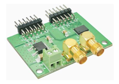
ADC module features AD9283 an 8-bit monolithic sampling analog-to-digital converter with an on-chip track and hold circuit. The maximum conversion rate is at 100 MSPS, with outstanding dynamic performance over its full operating range. This module is designed to be used with Numato Lab's FPGA/Micro-controller boards featuring a 2×6 pin Expansion connector. It can also be used with other boards and connector types by using manual wiring.
