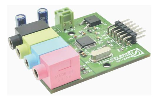
AC'97 Rev 2.1 compliant audio codec which enables producing and recording high-quality stereo audio. This module is designed to be used with FPGA/Microcontroller boards featuring a 2×6 pin Expansion connector. It can also be used with other boards and connector types by using manual wiring. This product is compatible with many Numato Lab's FPGA boards.
