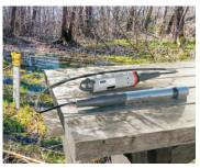
HOBO MX800 Series wireless data loggers work with interchangeable sensors to provide a highly configurable solution for monitoring water conductivity/salinity, temperature, level, and dissolved oxygen (coming soon). Available in both an easy-to-deploy, fully submersible model (MX801) and a direct read model (MX802) for convenient data offload that doesn't require having to remove sensors from the water.
