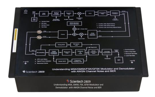
**Scientech 2809** is an ideal platform to study & experiments different topics like Minimum Shift Keying (MSK), Gaussian Minimum Shift Keying (GMSK), Frequency Shift Keying (FSK), Gaussian Frequency Shift Keying (GFSK) etc. which are the part of the Continuous Phase Frequency Shift Keying technique. Scientech 2809 also includes the study of AWGN noise & BER measurement. Built-in data acquisition system will help user to analyze the signals using real-time software.
