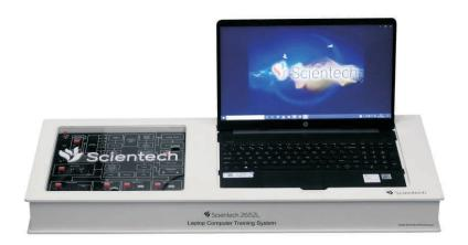
Scientech 2652L Laptop Computer Training System is a versatile product to provide training on hardware and software of a Laptop Computer. This is based on Intel® Core™ i3 with integrated Intel HD Graphics with experiments on Windows operating system.
