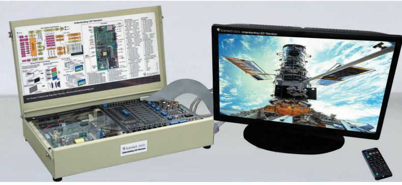
**Scientech 2651A Understanding LED Television** is a friendly training platform to learn the operation of LED Television receiver. It is demonstrator cum training system specifically designed for the comprehensive practical study on LED TV engineering for the beginners with a basic knowledge of the various electronic building blocks and fundamentals of communication system.
