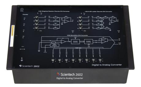
**Scientech 2602** Digital to Analog Converter composed of devices that transform a digital word into analog signal. The Digital to Analog Converter
