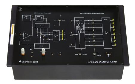
**Scientech 2601 Analog to Digital Converte**r composes of the devices transforming an analog signal into discrete signals. It converts continuously varying signal with time into discrete signal. The Analog to Digital converter Scientech 2601 TechBook demonstrates two techniques :
