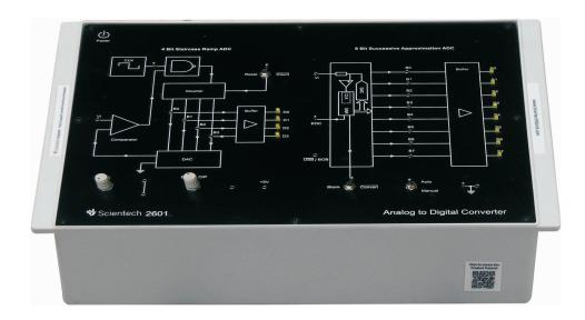
**Scientech 2601 Analog to Digital Converte**r composes of the devices transforming an analog signal into discrete signals. It converts continuously varying signal with time into discrete signal. The Analog to Digital converter Scientech 2601 TechBook demonstrates two techniques:
