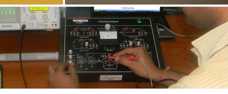
**Scientech 2321 Transistor Analyzer** provides the facilities for Transistor Static Test and Curve Tracing. These two are generally the most conventional tests used in laboratories. It is designed to show the complete arrangements of all the test methods and procedures. Scientech 2321 is a comprehensive solution for study of Transistor Testers and Testing of Transistor both. It supports both NPN and PNP transistors.
