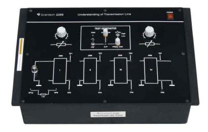
In the telecommunication field transmission lines are used to convey the signals from one point to another. The line properties become very important specially in multi-channel systems. Scientech Transmission line trainer Scientech 2266 is unique in design for experimenting various properties of the line. The trainer provides basic concept of coaxial line and include devices and accessories to conduct the experiment.
