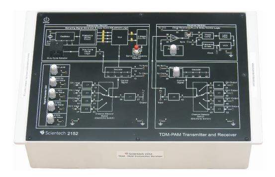
**TDM-PAM Transmitter and Receiver Scientech 2152** is a communication system where the message signal is modulated using Pulse Amplitude Modulation and multiple access is provided using Time Division Multiplexing. The message information is encoded in the amplitude of a series of signal pulses and transmitted using Time Division Multiplexing (i.e. in different time slots).
