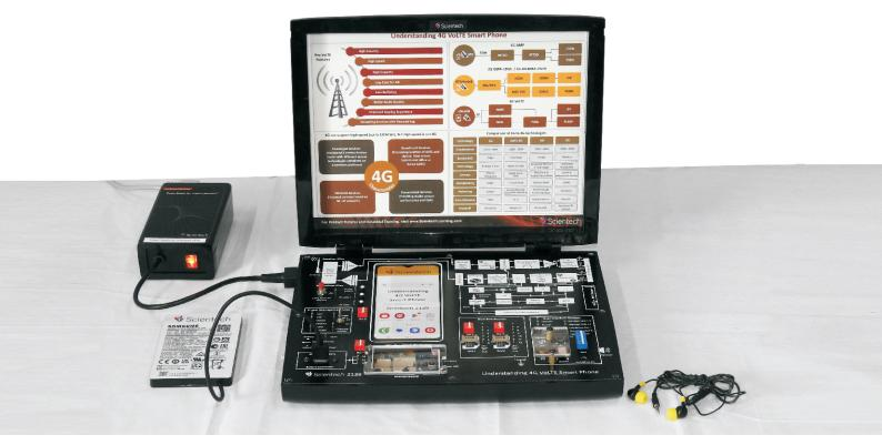
**TechBook Scientech 2139 Understanding 4G VoLTE Smart Phone** is a unique, self contained, easy to operate, training and platform that demonstrates the complete study and working of a 4G Dual SIM VoLTE handset to understand the fundamentals of Smart phone.
