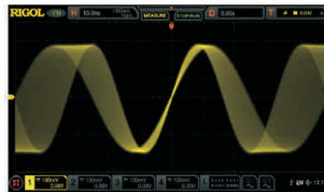
Changes of each frame of waveforms of the sweep signal can be clearly observed in the highly refresh mode.
