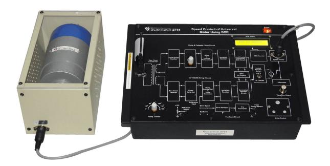
**Scientech 2714** is a platform which is very useful for Students to understand the concept of Thyristor firing method & working of speed control of motor using SCR by two different firing method. This platform is provided with inbuilt power isolation circuit to observe the high voltage output signal on Oscilloscope. This platform is provided with inbuilt AC/DC power supplies & exhaustive learning material.
