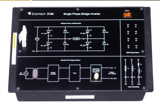
**Scientech 2720 Single Phase Bridge Inverter** has been specifically designed to understand the working of Bridge Inverter with various load configurations. It also helps the Students to understand the working of SCR firing fundamentals.
