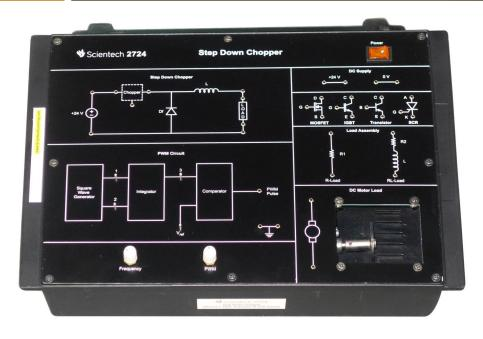
**Scientech 2724** is a learning platform which is very useful for Students to understand the concept of DC to DC chopper on various load configurations. 2724 is provided with various devices like MOSFET, IGBT, Transistor & SCR.
