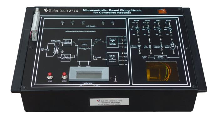
**Scientech 2716** is a learning platform which is very useful for Students to understand the concept of Microcontroller based thyristor firing method & working of single phase controlled rectifier on various load configurations. Scientech 2716 is provided with inbuilt AC/DC power supplies & exhaustive learning material.
