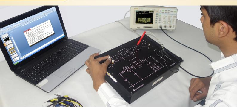
Scientech 2726 is a compact and user friendly learning platform which is very useful for students to understand the concept of PWM generation technique, and Buck Converter topology on various load configurations. It is also helpful for understanding the converter output on various filter configurations. Platform explains PWM generation technique, Buck converter operation, and power isolation circuit to measure the isolated output.
