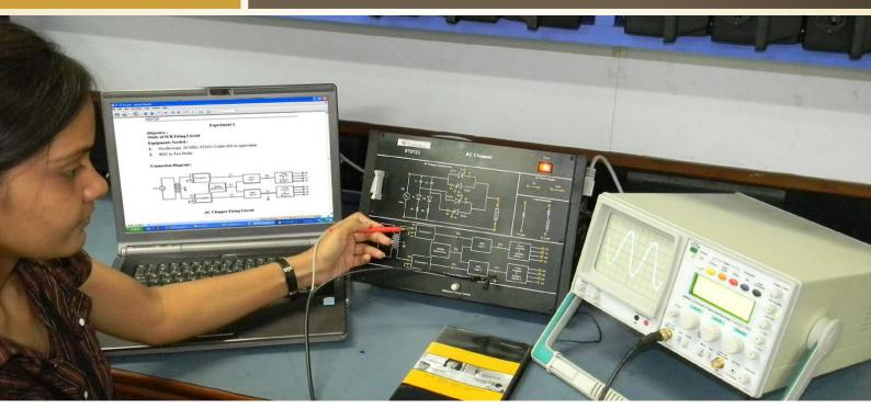
Scientech 2723 is a learning platform which is very useful for Students to understand the concept of thyristor firing method & the working of AC to AC conversion on various load configurations. Platform is provided with inbuilt DC power supply & exhaustive learning material.
