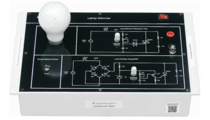
**Scientech 2711** is a comprehensive learning platform which is very useful for Students to understand the application of Thyristor in intensity control. Two firing methods are provided with this platform internal power attenuattor is included for observation of high voltage signals on the Oscilloscope. This platform is provided with internal AC/DC power supplies & exhaustive learning material.
