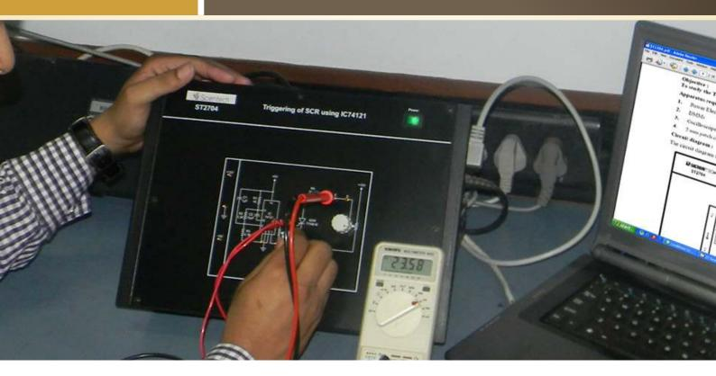
**Scientech 2704** is a platform which is very useful for Student to understand the thyristor triggering by using monostable multivibrator. 2704 is provided with in built Power Supply, sockets for making interconnections in the circuit and exhaustive learning material.
