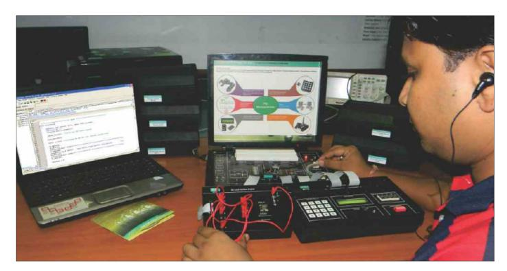
Nvis Technologies SD card interface module, MC14 is an extension module for Nvis Microcontroller development platforms. The object is to have a clear understanding of how Industry Standard SPI communication based SD card can interface and controlled with Microcontroller.
