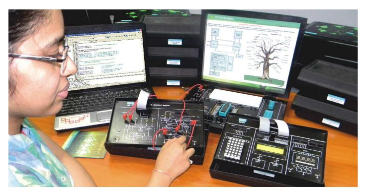
I<sup>2</sup>C protocol based ADC/DAC module enables students and practicing engineers to gain practical experience of applications of Microcontroller. The object is to understand how two wire serial interface device is used for interfacing with Microcontroller to communicate with external applications. Analog inputs are converted into digital through Microcontrollers and vice versa. ADC/DAC module, has input and output terminals for connection of external real world applications.
