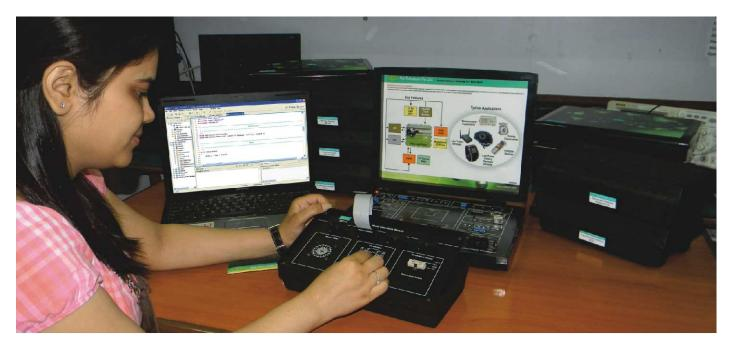
Nvis Technologies Multi interface module MC11 is an extension module for Nvis Microcontroller development platforms. The object is to have a clear understanding of how input peripherals are interfaced and controlled with Microcontroller. MC11 has been designed to have a clear understanding of how Stepper Motor is interfaced and controlled with Microcontroller. It also gives a clear understanding of SPI and I<sup>2</sup>C interface bus for data transfer.
