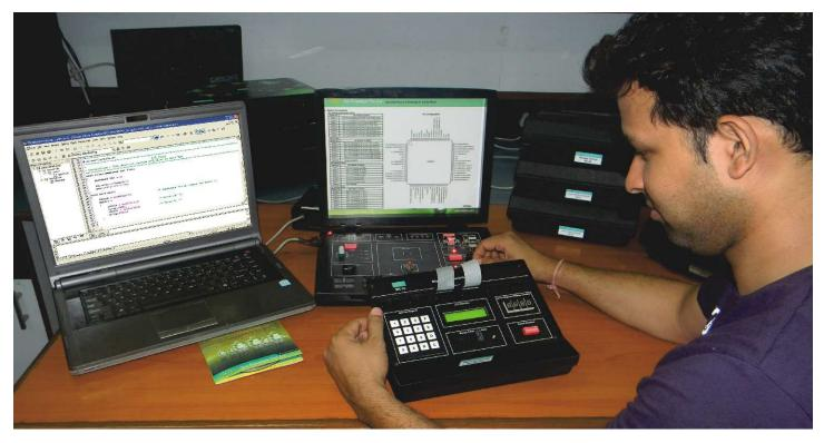
**Nvis Technologies Display and Switches module MC10** is an extension module for Nvis Microcontroller development platforms. The object is to have a clear understanding of how input peripherals are interfaced and controlled with Microcontroller. The object is to connect and program a Microcontroller to display data and for monitoring.
