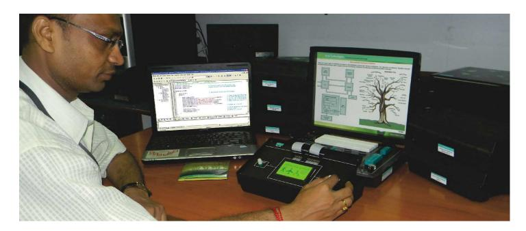
Graphical display module MC09 helps the user to gain invaluable practical experience of the principles and application of Graphical LCD display in Microcontroller based projects.
