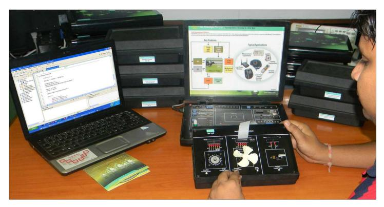
Motor Drive module MC05 is an extension module for Nvis Microcontroller development Platforms. MC05 has been designed to provide a clear understanding of how motors are interfaced and controlled with Microcontroller. The Motor Drive module is made in such a way that student can understand the detailed concepts of Stepper Motor, DC Motor, and Servo Motor system.
