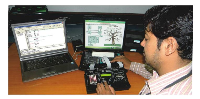
**Display module MC04** is a learning platform to study the working of displays used for industrial applications. MC04 has been designed to demonstrate the applications of Nvis Microcontroller development platforms. The object is to connect and program a Microcontroller to display data and monitoring. Contrast and backlight control are provided on the module.
