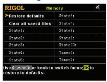
It supports storing and recalling state files and timer files, and allows you to restore the instrument settings to defaults.
