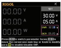
You can set thresholds for OVP and OCP values. If overvoltage or overcurrent occurs, the power supply shuts down the output automatically, and then a prompt message is displayed.
