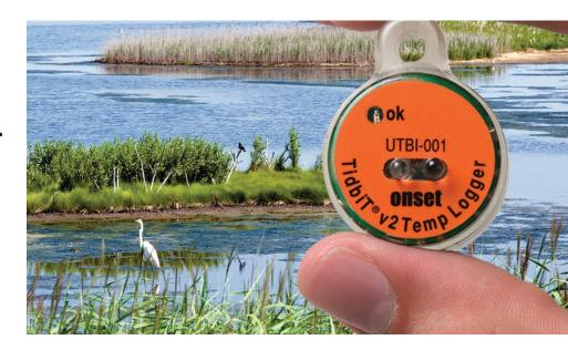
Onset's smallest data logger, the TidbiT v2 has 12-bit resolution and a precision sensor for ±0.2°C accuracy over a wide temperature range. It is waterproof to 300 meters (1,000 feet) and can be used in a wide range of water temperature monitoring applications.
