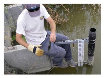
A high-accuracy, cost-effective data logger that measures and records conductivity and temperature in streams, lakes, and other freshwater sources. Recommended for monitoring aquifers for saltwater intrusion and road and agricultural runoff, this logger's open access to its sensor simplifies cleaning and maintenance, and its non-contact sensor minimizes measurement errors related to drift. Also features software-based drift compensation.
