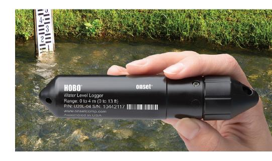
The HOBO U20L series loggers are lowcost, research-grade water level data loggers for continuously measuring water level and temperature in a wide range of underwater environments. They feature 0.1% measurement accuracy, a polypropylene housing for use in both fresh and salt water, and a non-vented design for convenient and hassle-free deployment.
