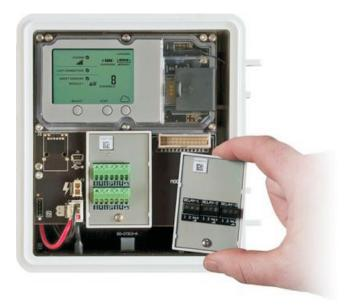
An optional analog module with four analog inputs that support excitation power, scaling, and statistics measurements. These four, single-ended sensor inputs are configured through HOBOlink. A HOBO RX3000 is required for this product.
