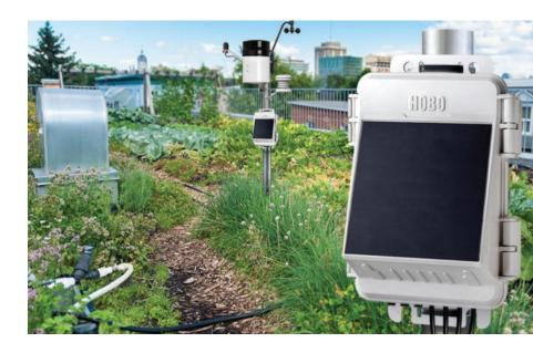
The new web-enabled HOBO MicroRX station is an easy-to-deploy, low-cost cellular field monitoring solution. With a compact size and rugged design, the MicroRX Station offers long-term, reliable environmental monitoring. Configurable station-side alarms provide immediate notification of critical conditions, and Onset's cloud-based HOBOlink platform makes it easy to view, access, and share your data.
