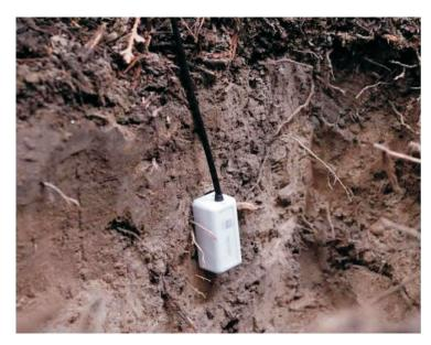
Low-cost, fully integrated soil moisture loggers with Bluetooth wireless data offload. Available in two models – one that measures soil moisture (HOBO MX2306) and one that measures both soil moisture and temperature (HOBO MX2307) – these loggers are ideal for researchers and growers looking for the accurate data they need to save water, improve crop yields, reduce harmful runoff, and protect ecosystems.
