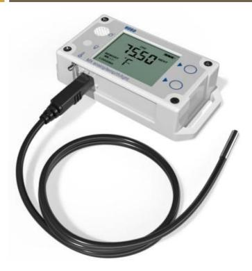
Makes it easy to monitor four measurements with one versatile logger. The kit includes the HOBO MX1104 logger with integrated sensors for temperature, humidity, and light, plus an external temperature sensor with a 6' cable. This is a great addition to your toolbox for troubleshooting, equipment scheduling, building commissioning, HVAC performance monitoring, and more! The external input provides the flexibility to connect a wide range of sensors, expanding monitoring capabilities.
