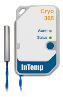
The InTemp CX703 Cryogenic data logger is a low-cost Bluetooth-enabled multiple-use logger that records temperature data for up to 365 days. The CX703's built-in 1.5m probe measures temperatures as low as -200°C (-328°F) and includes a protective sheath to prevent accidental cutting of the cable.
