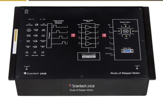
Scientech 2458 Study of Stepper Motor explains students the operation and control of Stepper Motor effectively. It helps the student in understanding half and full step angle of Stepper Motor. The LED's provides the visual indication of the coil excitation process. It has a provision for connecting the motor with an external controller. Stepper Motor are widely used for application such as Conveyor system, Robotics, Printing machine, Solar tracking system, Elevator load etc.
