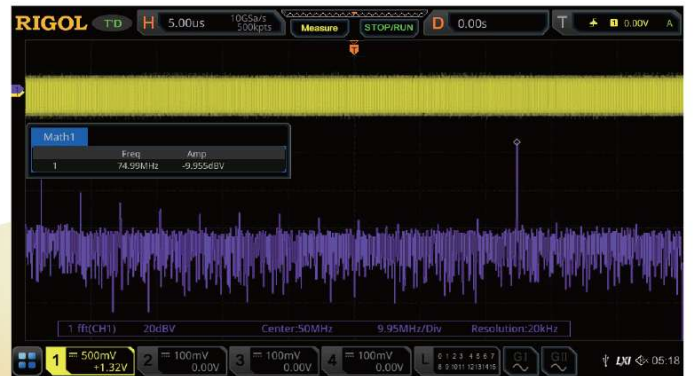
With the near-field probe, you can easily observe the spectrum peak in the frequency domain when the probe approaches to the radiation leakage point.
