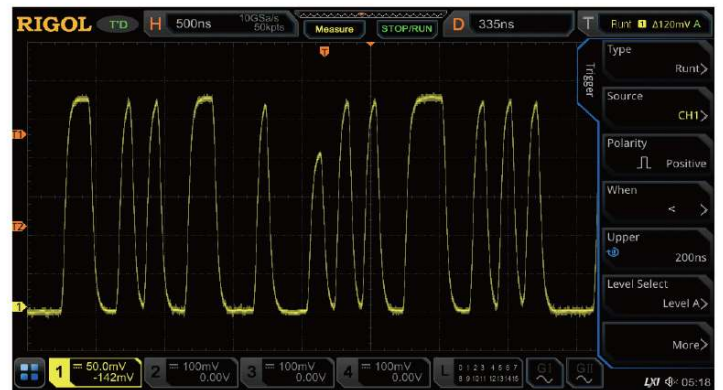
The Runt trigger helps you capture the runt pulse signal in the pulse train
