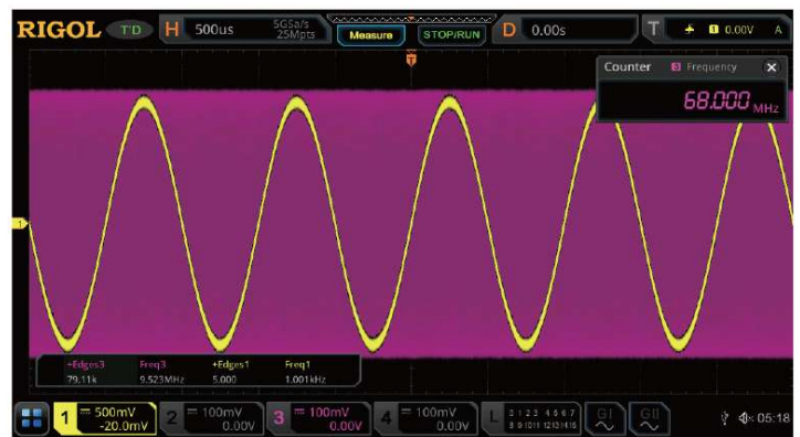
The ordinary 1 Mpts software measurement can no longer measure the accurate frequency of the high-frequency signal.
