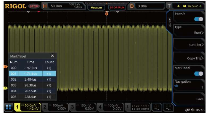
The search and navigation function can quickly search for the signals with exceptions and locate them accurately.
