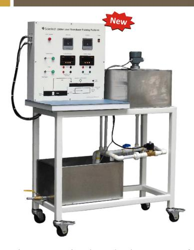
Scientech 2309M Level Transducer Test Bench is designed to learn concepts of water level measurement. It helps students & industry professionals to understand operation of level sensors in detail Scientech 2309M level Transducer Test bench includes different types of level transducers including, capacitive level transducer, float switch, ss sump tank and measuring tank, pump, solenoid valve, voltmeter, ammeter and 4-20mA current and 0-10VDC voltage display.
