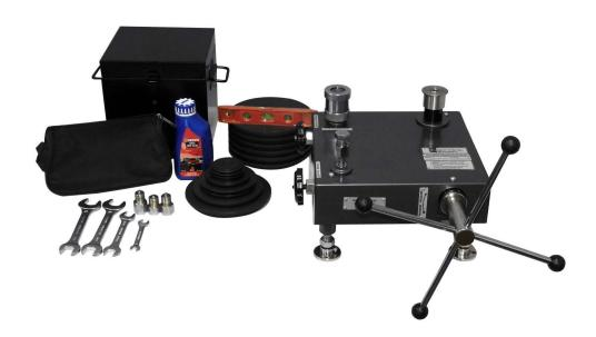
**Scientech 2434T Dead Weight Tester (DWT)** is an instrument that is used to calibrate pressure gauges. It basically works on the pressure balance principle with calibrated weights used to apply pressure to an area. When the pressure balance reaches zero, the pressure device under test is considered calibrated. DWT provides high accuracy in pressure gauge calibration and prevents the occurrence of an error in pressure reading.
