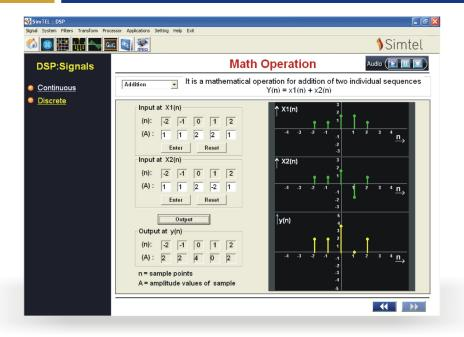
The Simtel DSP module is unique software to understand the concepts of Digital Signal Processing. This is a good tutorial to learn the basics of DSP in an easily understandable way without resorting to too much Mathematics. It offers real time understanding of DSP algorithms and a better visualization of signals and their applications through simulation. Graphically based programs provide easy understanding of DSP hardware and applications.
