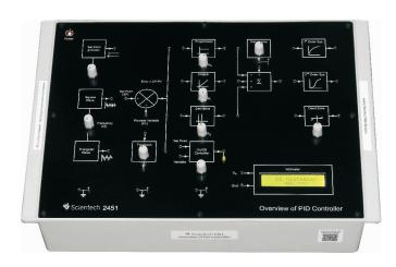
In Control System there are different types of Controllers. Study of two-position mode as ON/OFF Controller and continuous Controller modes as PID controller is a very important part of control engineering. To have a basic idea and practical hands on Controllers PID Scientech 2451 has been designed to be used by students to investigate the principles of PID by applying different signals.
