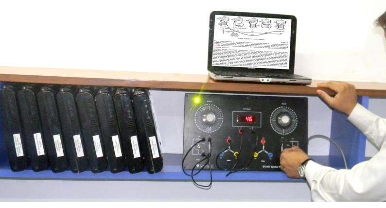
Scientech 2455 Synchro Transmitter and Receiver helps the users to gain invaluable knowledge about the working principal and operation of Synchro motors. Onboard AC voltmeter to measure the voltages between rotor and stator windings are also available.
